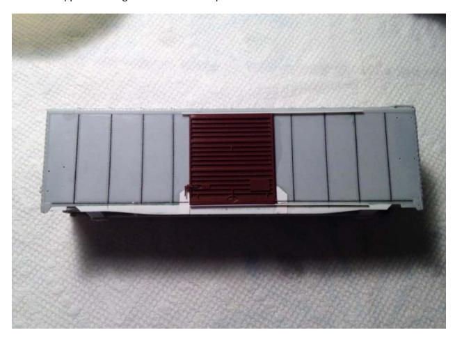
Once the welds are dry, glue on the door stops that were saved in the beginning at the ends of the door tracks.
